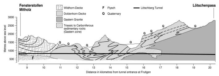
Fig. 2. Geological cross-section of the northern part of the Lötschberg base tunnel, based on web data published by the BLS-AlpTransit Geologists on November 6, 2006.
