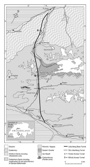
Fig. 1. Tectonic map of the study area, modified after Kellerhals and Isler (1998). The position of the profile shown in Fig. 2 is marked on the Lötschberg base tunnel axis (A-B).
