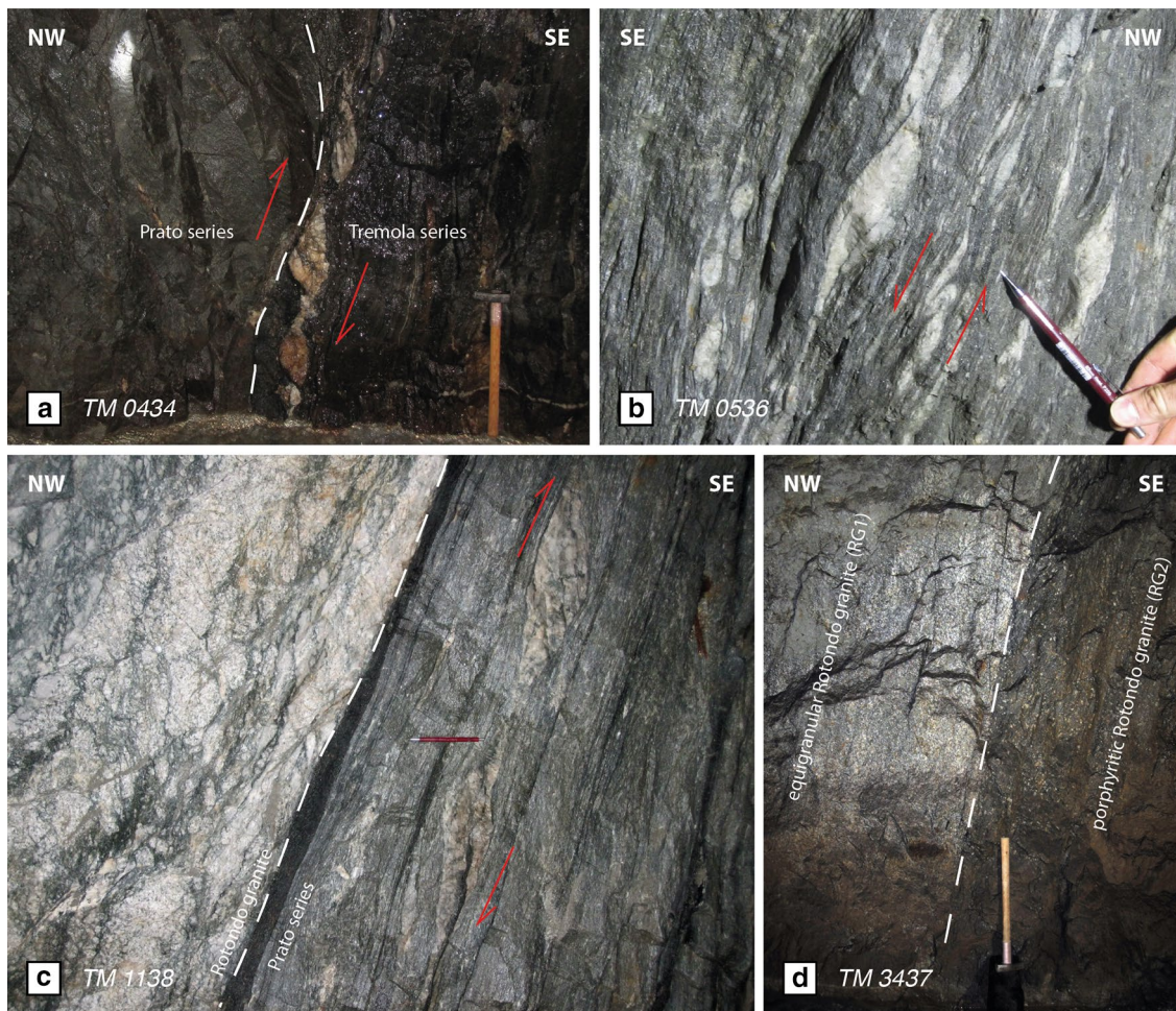
Fig. 5 Field photographs. Italic numbers correspond to tunnel meter (TM) where the images were taken. This is also valid for subsequent figures with field photographs or photomicrographs and will no longer be mentioned. a Contact between Tremola series in the SE and Prato series in the NW, hammer for scale. b Folded and sigmoidal quartz aggregates indicating top-to-south shear sense (upward movement of the northern block) in the Prato series, pencil for scale. c Contact between Prato series in the SE and Rotondo granite in the NW. The Rotondo granite consists at the contact to the Prato series of an approximately 5 m wide zone of highly deformed granite. Pencil for scale. d Contact between the porphyritic variety of the Rotondo granite (RG2) in the SE and the equigranular variety of the Rotondo granite (RG1) in the NW. Note that the RG2 is relatively strongly sheared at the contact and that the RG2 further to the SE is not as dark as in this photograph. Hammer for scale
