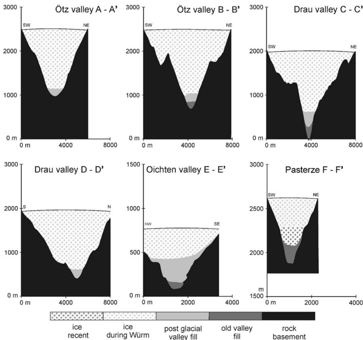
**Fig. 11** Representative cross-sections of Ötz-, Oichten-, Drau Valley and Pasterze glacier. Ice cover during ice age, recent glacier ice, post glacial sediments, old valley-fill, and rock base are assigned by grey scales (see legend)
